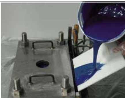
Pouring from lowest corner
