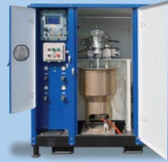
Automatic paint blending equipment
